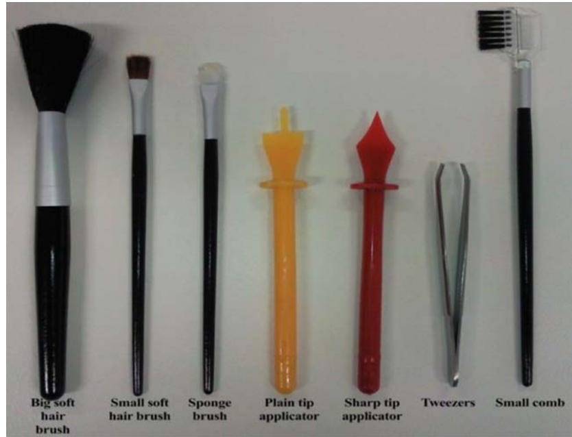
Figure 1. Toolset used for manual picking and fixation of yarn hairs on paper base.
